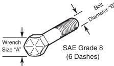
Proper toque for American fasteners used on Bush Hog equipment. Recommended Torque in Foot Pounds (Newton Meters).\*
