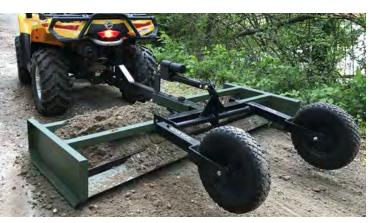
The Bush Hog® ATV/UTV Terra Hog System starts with a strong tubular steel frame. Each frameconsistsofyourchoiceofeitheramanual ratchet jack or electric actuator to raise the wheels out of the way when in use. Each frame will accommodate 10 different implements to help you get virtually any job done. **Choose from:**
