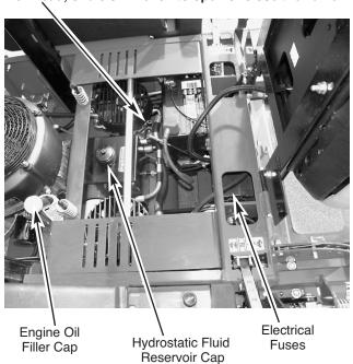
NOTE: To move the tractor without power, the pumps must be unlocked and in the free wheel position. Failure to do so could possibly damage the hydraulic motors. Never pull at more than 2 MPH.
