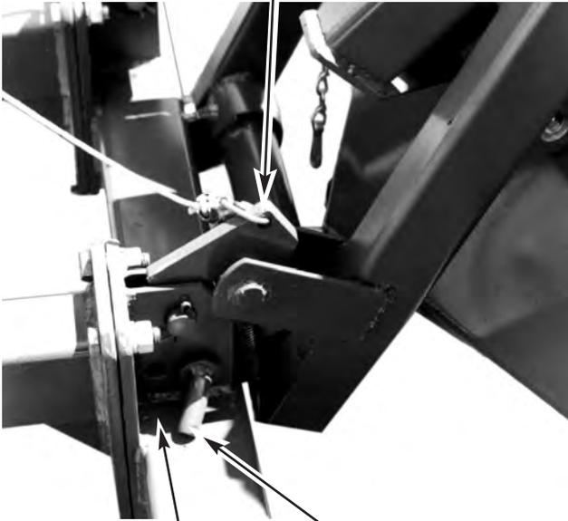
Transport Lock Hole      Pin In "Working" Position
