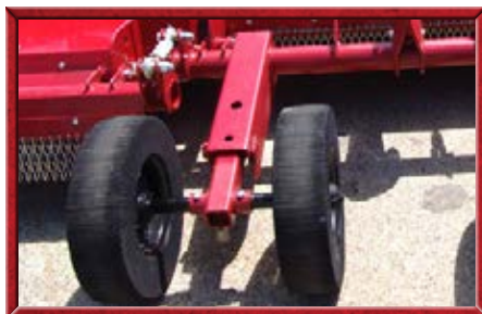
Each axle arm on the center section has a rubber cushion to absorb the shock loads near the wheel.
