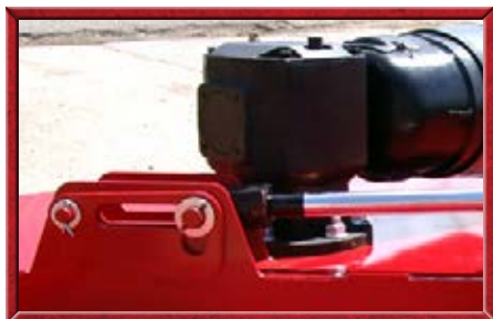
Wing free float is 22° down and 25° up without movement of hydraulic cylinder rod for extended cylinder life.
