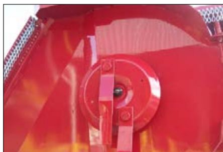
The design of the wings adds exceptional strength in the gearbox stands without the use of exposed structure.
