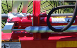
Each rake wheel has a spring for flotation. Final rake wheel pressure can be adjusted by use of crank adjustment.
