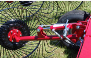
Front finger wheels can be adjusted upward to convert to an 8 wheel rake. Either side can be raised to form windrow to right or left.
