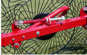
Independent wheel suspension allows for minor adjustments of each wheel to ensure top performance of hay movement in rough or uneven hay fields.
