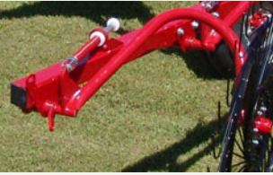
Front finger wheels can be adjusted upward to convert to an 8 wheel rake. Either side can be raised to form windrow to right or left.
