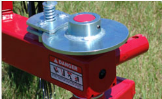
Adjustable wheel brake stops gauge wheels from shimmying in field and during transport.
