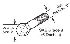
Proper toque for American fasteners used on Bush Hog equipment. Recommended Torque in Foot Pounds (Newton Meters).\*
