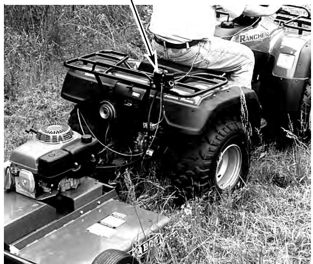
Figure 2-4 Control Box Mounted On ATV Rack
