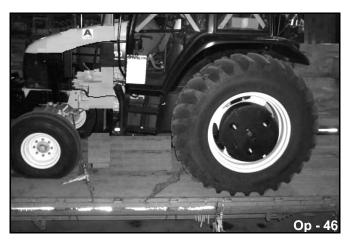
Use adequately sized and rated trailers and equipment to transport the tractor and implement. Consult an authorized dealer to determine the proper equipment required. Using adequately sized chains, heavy duty straps, cables and/or binders, securely tie down both the front and rear of the tractor utilizing the proper tie down locations as specified by the tractor manufacturer. *OPS-U-0025 str*
