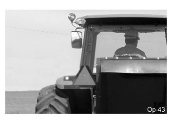
Make sure that all tractor flashing warning lights, headlights, and brake/tail lights are functioning properly before proceeding onto public roads. While newer model tractors have plenty of lighting to provide warning signals and operating lighting, most older models are only equipped with operating lights. Consult an authorized tractor dealer for lighting kits and modifications available to upgrade the lighting on older tractor models. *OPS-U- 0021str*
