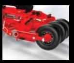
Custom-tuned rubber isolator pads absorb shock at each axle
