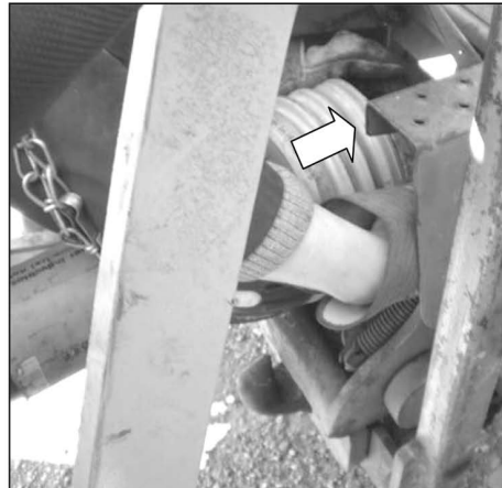
Attach PTO shaft to the output shaft of the tractor.
