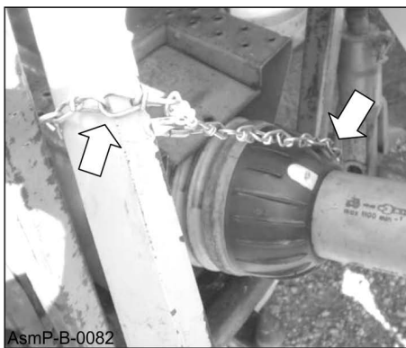
Attach torque chains to convenient locations to prevent rotation of PTO shaft guarding.
