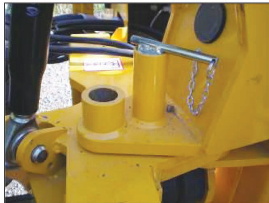
Slew Unlocked – only for working
