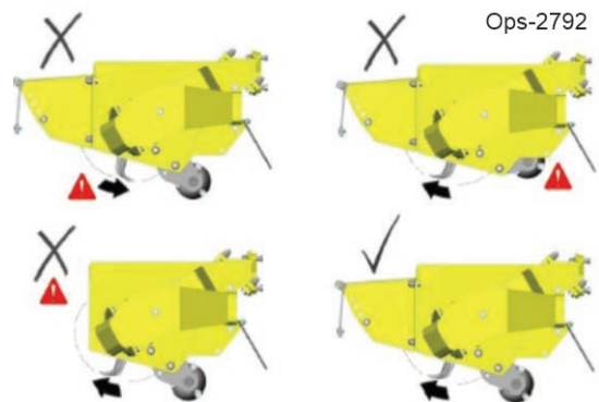
Ops-2792 When mowing grass always cut in the uphill direction with front hood fitted and roller positioned below cutting height of the flails.
