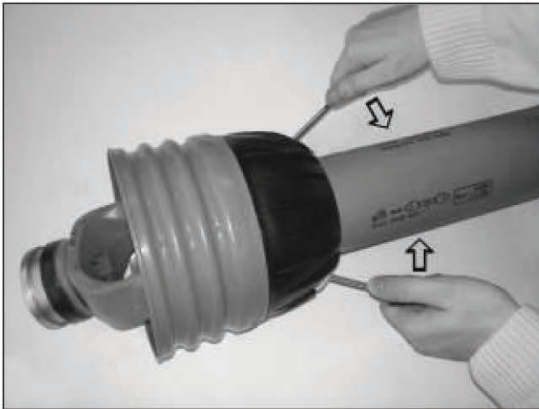
Prise clasps open to release the shield
