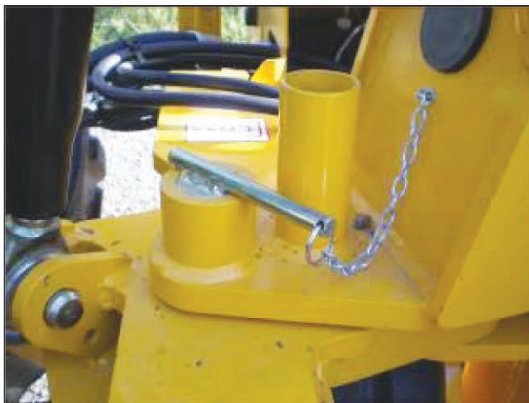
Slew Locked – always for transport & storage
